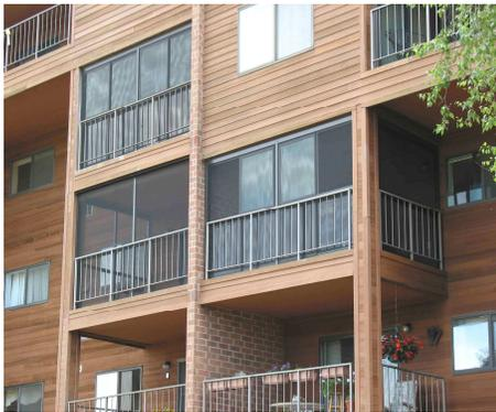
Our special design allows the panels to be easily installed from the inside. Great for highrise balconies. Roofing systems to be contractor constructed.
